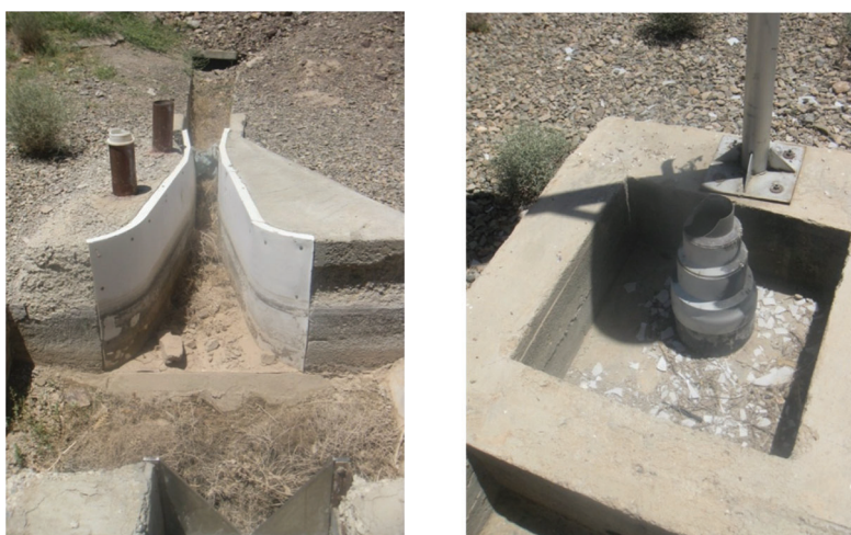
Figure 17. Inappropriate maintenance of installed instruments in Izadkhash dam, Weir (left) and Piezometer (right)
